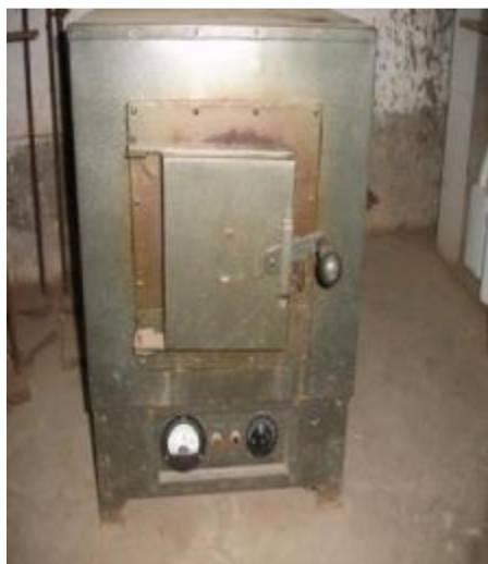
Photo 3 ) Ashed in a muffle furnace at 500 0 c for 2-3 hours.
