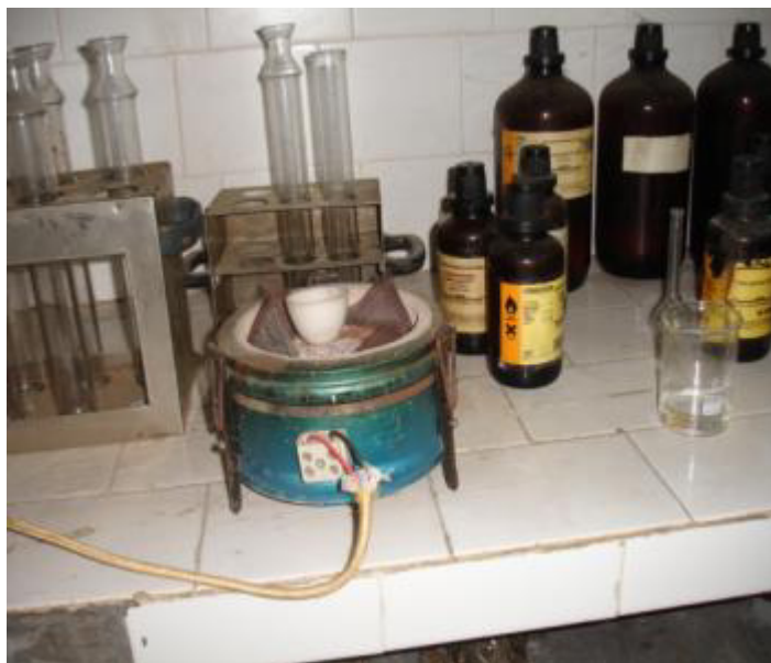
Photo 2 ) A small amount was taken with a spatula in a crucible, weighed and charred in a electric heater for about 1 hour.
